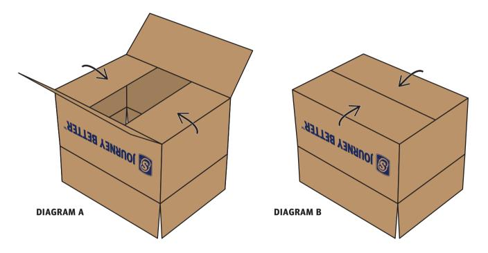
**4.** Using the tape machine, position the tape scale to #22 and pull the handle to release 20" (50.80cm) of branded tape.
