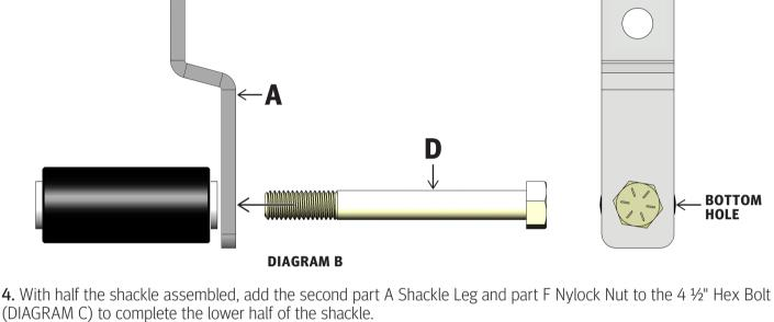
bottom hole of the shackle leg and rollers (DIAGRAM B).
