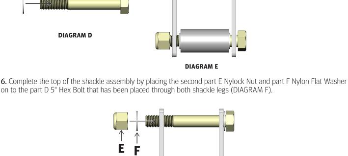
7. Finish the completed shackle by placing a part G Do Not Tighten Sticker at the top of the leg of the shackle next
