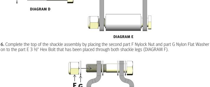
**DIAGRAM F** 7. Finish the completed shackle by placing a part H Do Not Tighten Sticker at the top of the leg of the shackle next
