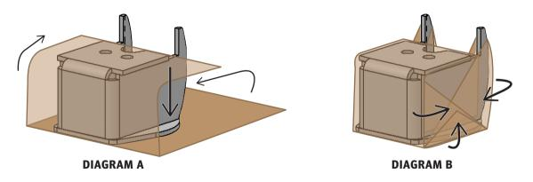
**16.** Place the SumoSprings inside the box (refer to diagram below), both need to be in the same direction of each other and packaged to the left side of the box. Place the brackets to the right side of the box. Using the filler paper machine, release enough paper to fill the space it between the SumoSprings and brackets in the box and over the top of the bracket bundles. The SumoSprings and brackets should fit snug with little to no movement.
