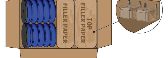
17. Place the 7" (17.78cm) bag with the accessories in the box, between the SumoSprings and brackets.
